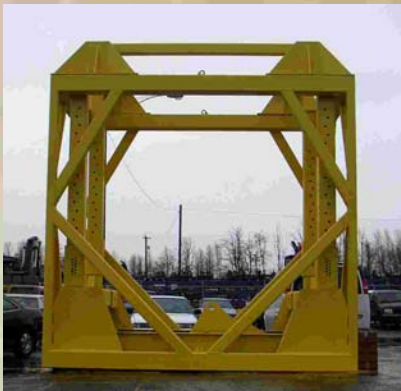
FORESTRY CAB TEST STRUCTURE
